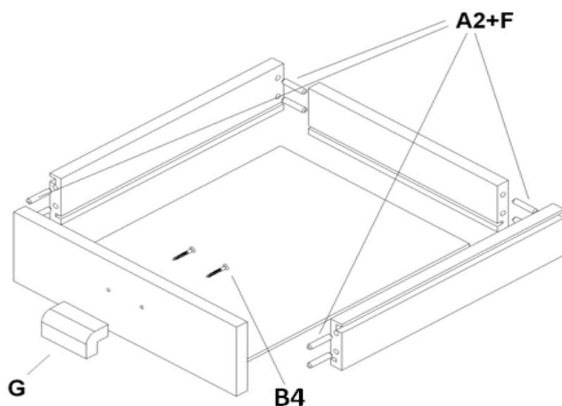
**!!! HINT 1 !!!** - Do not fill dowel holes with glue. Smear the dowels and the surfaces of the wooden parts with glue and insert them into the holes.
