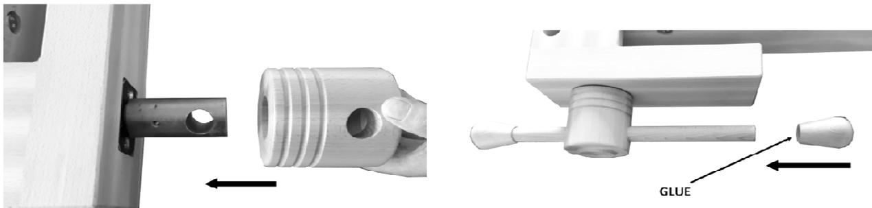
**Hint.:** Smear inside knob as well as wrench by glue and put together. Wipe off excess glue with a cloth.
